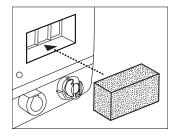
Installing the Filter
