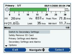
**Note:** In the Options menu described later in this chapter, you can specify the Pressure Units displayed by the device, choosing either cm  $H_2O$ , hPa, or mBar. The default setting is cm  $H_2O$ , so this manual uses cm  $H_3O$  throughout.
