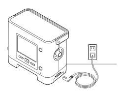
**Note:** This device is activated (i.e., 'powered on') when the AC power cord is connected or any of the three battery sources is available. Pressing the Start/Stop button turns the airflow on or off.
