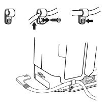
Securing the Power Cord Using the Cord Retainer
