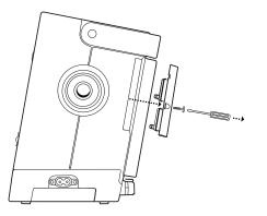
Unscrewing the Exhalation Porting Block 2. Using the flat side of the screwdriver, pry the exhalation porting block away from the device until it comes loose, as shown below.
