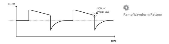
For the active circuit in volume modes, peak flow is required to be a minimum of 20 l/min. The wave form may be flattened when the combination of Inspiratory Time and Tidal Volume set points would result in a flow of less than 20 l/min. Therefore, for some settings, a Ramp flow pattern may provide a pattern that more closely resembles a Square flow pattern.
