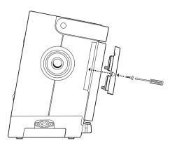
Installing a New Exhalation Porting Block
