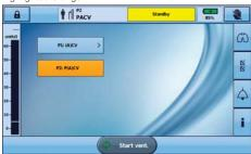
Note: To change to a program with a different circuit type, you will need to stop ventilation. When you have changed the circuit and the program, you can restart ventilation.
